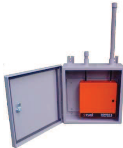
Figure 1AR-3 Repeater in ES161606-FR2 Enclosure with One Short Sheath
